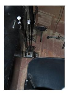
There are two control levers on the Motorcar: a 'Lockout' lever on the left and a 'Shift Lever' to its right.
